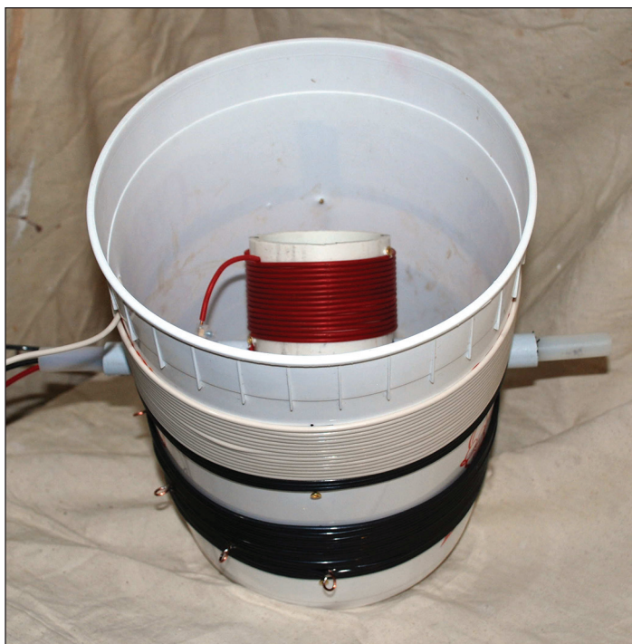
Figure 5: Homebrew variometer inside main loading coil. (courtesy VA7BBG)
