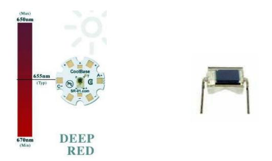
The LED is a Luxeon Red Rebel mounted on a 'Star' base and then on to a small heatsink. The LED operates @ 700ma for ~ 1.5W input. The receiver's PIN Photodiode is BPW34 (about 3mm square) that is spec'd for 430-1100nm. At 655nm, it performs at 60% efficiency compared to 1100nm so our system should work even better in IR but will make aiming more difficult.
