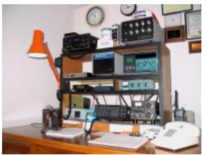
Kenwood 570S (HF all band +6M) inc Kenwood PS-30 Power Supply Kenwood AT-180 Antenna selector and tuner plus SWR meter
