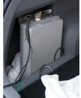
new vehicle, the lead from the tuner to the base of the antenna was about 24", so I decided that what was needed was a piece of shielded coax, which is ground at both ends. I proceeded to install this and then tried the little baby out, and lo and behold, no more lit up dashboard and the tuner was able to tune in the hf bands with no problem, so the problem was solved. I'm a happy
