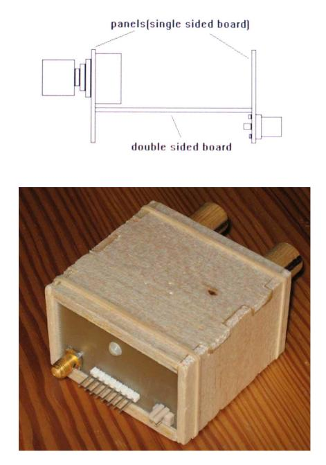
The case is made from balsa wood sheet. Three pieces of sheet are made into a U-shape, into which the chassis is dropped. A fourth sheet drops in on top as a lid. Both the U and the lid have small pieces of balsa glued to the inside which engage the rear panel to stop the chassis from sliding back and forth. This lid is held on simply by wrapping a couple of elastic bands around the whole rig; it's not very elegant but I haven't thought of a better way.
