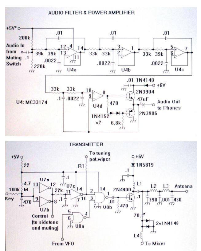
U7: 74C04 U8: 74HC02 All Inductors #30 AWG enamelled wire. L1: 26 turns on FT23-43, L2 & L3: 18 turns on T37-6, L4: 50 turns on T37-2.
