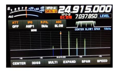
The screen should look more like the following one, where the audio level at the computer is increased only up to the point where the RF power output does not increase any further – in this case the ALC reading is near the middle of the white part of the meter scale.
