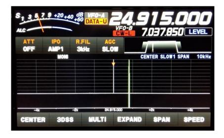
The following settings work for me for FT8/FT4/MSK144 and produce a clean signal (Note 6).
