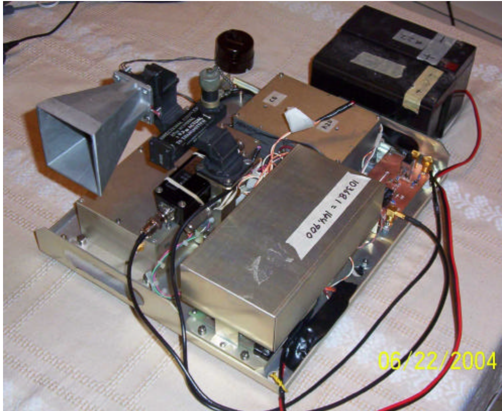
Figure 2: The modified transverter in the configuration used for its first QSO
