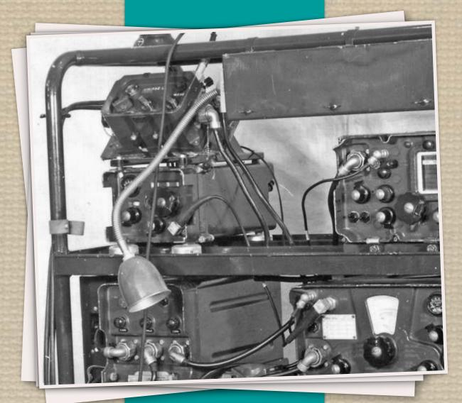
Small operator lamps were issued with most British (and Commonwealth) Army vehicle and ground radio stations, normally powered directly from a socket fitted on the front panel of the set. This overview shows the presently known versions and variations.
