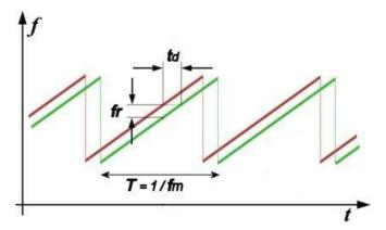
Fig. 6 - FMCW signals using Sawtooth waveform
