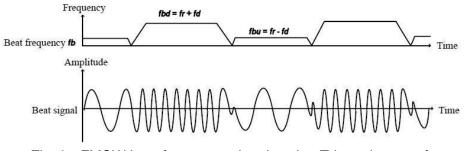
Fig. 3 - FMCW beat frequency signals using Triangular waveform
