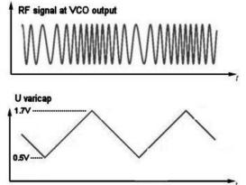
Fig. 8 - RF modulated signal at VCO output vs U varicap
