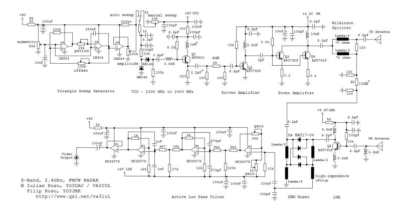
Fig. 16 - Schematic of the S-Band, 2.4GHz, FMCW Radar
