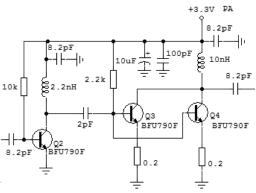
Fig. 9 - Power Amplifier schematic
