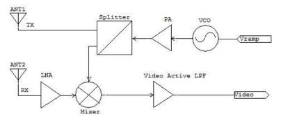
Fig.2 - Homodyne FMCW Radar Block Diagram
