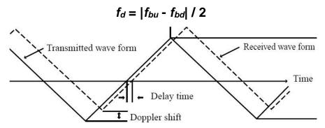
Fig. 4 - FMCW Doppler shifted received signal using Triangular waveform
