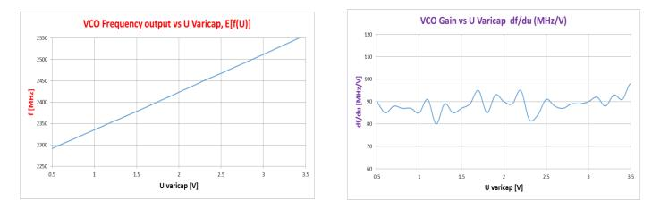
We can see from the above measurement's plots that the VCO which was built has more than 250MHz frequency range for a varicap voltage sweep between 0.5V and 3.5V. The actual project uses only 100MHz from this 250MHz frequency range. The chosen frequency range is between 2300MHz and 2400MHz (U varicap = 0.5V to 1.7V), region where the linearity characteristic of the VCO is reasonable, and also because this is a frequency band with less number of external interferers.
