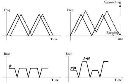
Fig. 5 – Effects of Doppler shift ( $f_d$ ) on beat frequency distance range ( $f_r$ )
