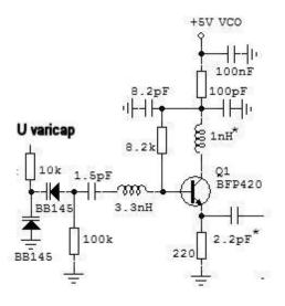
Fig. 7 - VCO Schematic
