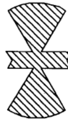
Shunt Radial Stub
