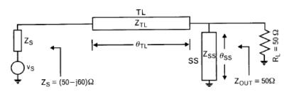
A complex source can be matched to the  $50\Omega$  load with a cascade series transmission line and a parallel short-circuited stub.
