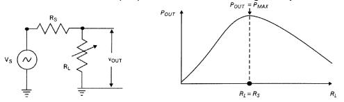
The circuit and graph to prove the condition for maximum power transfer
