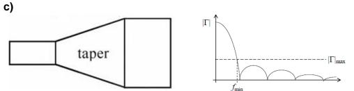
Another broadband matching approach may use a tapered line transformer with continuously varying characteristic impedance along its length (characteristic impedance varies continuously in a smooth fashion).
