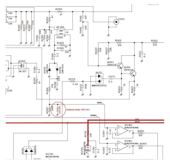
The best - experimentally found - value of the additional resistor is 100k Ohm. This value provides the practical matching range approx. SWR 1:6 (antenna impedance 8 to 300 ohm), that is much broader that originally.
