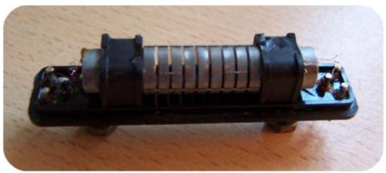
Carefully you have to unsolder the four thin wires that are coming from the transducers. Also have to unsolder the ground connections (one on each side). After that have to remove the rubber supports from the filter base. This is a very sensitive operation to don't damage the coupling wires that keeps together the metal disks.
