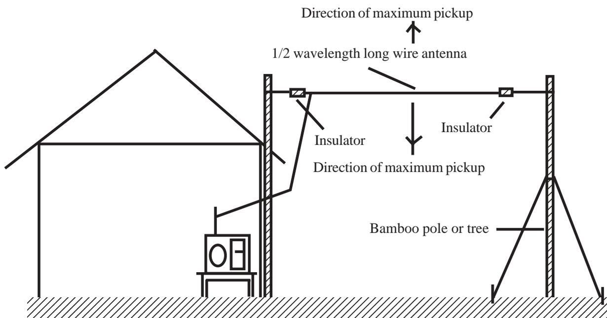
*An outdoor antenna is must to receive radio signals transmitted by ham radio operators. One end of the long wire may be simply connected to the telescopic rod antenna of the radio receiver*
