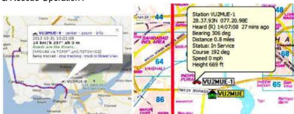
Figure 3: Real time plotting of mobile stations on internet as well as standalone computers connected to radio. Last reported time and position, bearing and distance from control room etc. are just at the click of a button.
