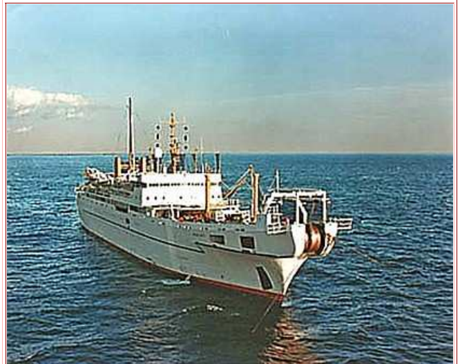
Cable Laying Ship CS Mercury Used on ANZCAN Project
