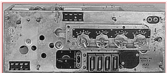
Photo 13 - VHF Transmitter Type BC625
