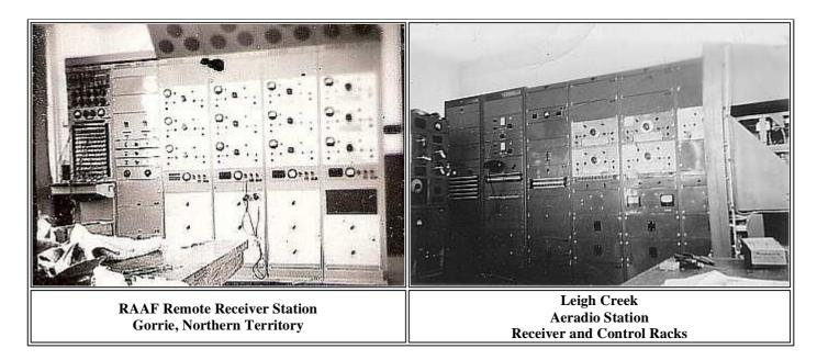
Not all of our AR7 receivers were modified for crystal locking or had Codans. A tuneable receiver was normally provided in the aeradio control console. The third picture shows the operating console at Leigh Creek with AR7 fitted and provided with all plug in coil boxes for continuous tuning (as original). Consoles of similar design (all built in our Parafield workshops) were also installed at Parafield and Mt. Gambier stations.
