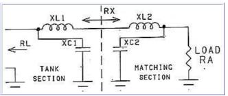
Figure 3: PI Network split into two sections for analysis.
