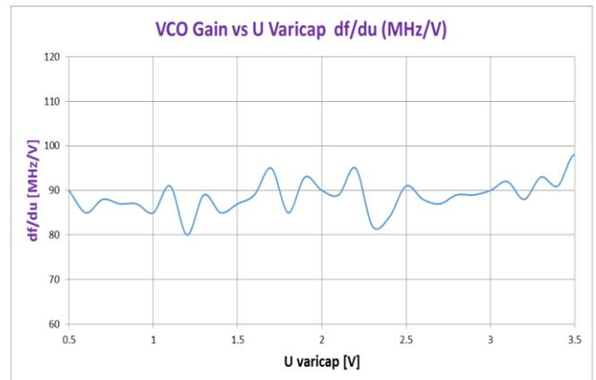
We can see from the above measurement's plots that the VCO which was built has more than 250MHz frequency range for a varicap voltage sweep between 0.5V and 3.5V. The actual project uses only 100MHz from this 250MHz frequency range. The chosen frequency range is between 2300MHz and 2400MHz ( $U_{\text{varicap}} = 0.5\text{V}$  to 1.7V), region where the linearity characteristic of the VCO is reasonable, and also because this is a frequency band with less number of external interferers.
