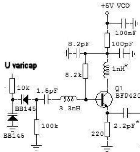
Fig. 7 - VCO Schematic
