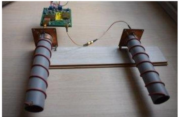
*Fig. 15 - Helical Antennas*
