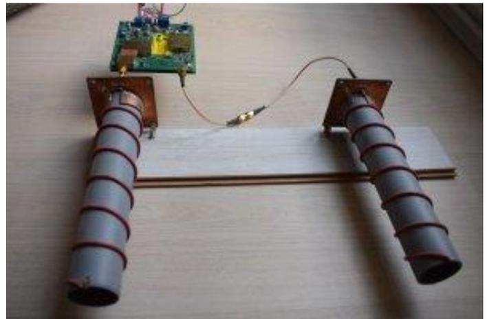
*Fig. 15 - Helical Antennas*
