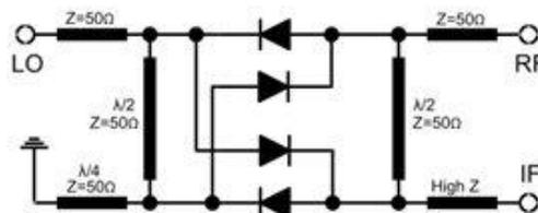
Fig. 11 - Planar Double-Balanced Mixer schematic
