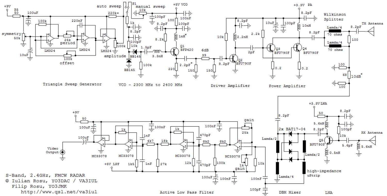
Fig. 16 - Schematic of the S-Band, 2.4GHz, FMCW Radar
