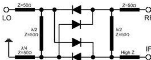
Fig. 11 - Planar Double-Balanced Mixer schematic
