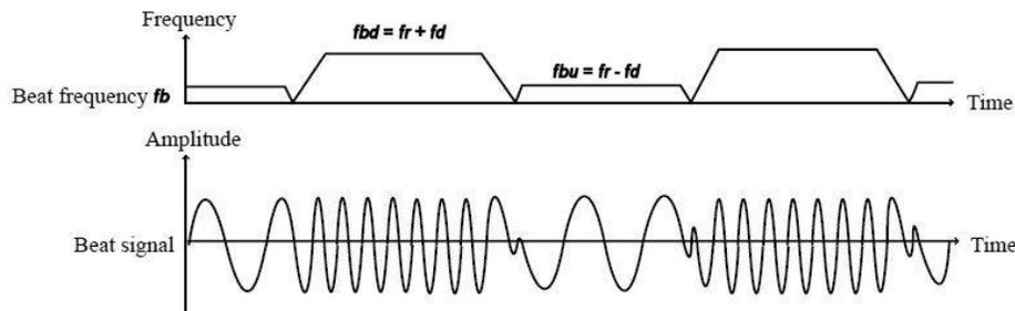
Fig. 3 - FMCW beat frequency signals using Triangular waveform
