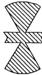
Shunt Radial Stub
