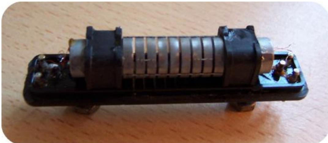
Carefully you have to unsolder the four thin wires that are coming from the transducers. Also have to unsolder the ground connections (one on each side). After that have to remove the rubber supports from the filter base. This is a very sensitive operation to don't damage the coupling wires that keeps together the metal disks.
