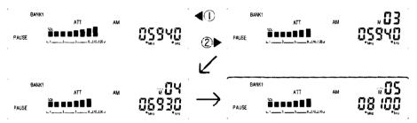
3 If you wish to continuously monitor a busy channel, you may temporarily disengage the pause scan mode by pressing [DIAL] once. To restart the pause scan mode press [DIAL] again.
