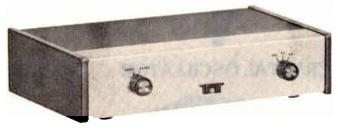
reduced a nominal 25%. Panel switch also selects the two transceiver crystal channels when fixed frequency use is desired. Includes cables (less crystals). **SPECIFICATIONS:** FREQUENCY RANGE: 1.8-2 MHz. SEN-SITIVITY: 1  $\mu$ V for 10 dB S+N/N max. RECEIVER FEED-THROUGH: -55 dB typical. POWER INPUT TO FINAL: 150 watts, approx. PANEL CONTROLS: 2 pos. band switch, 1.8-2 and 3.5-30.; 3 pos. mode switch, VFO, X1, X2. SEMICONDUCTORS: 1
