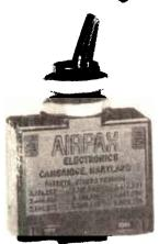
Model 1170 has operating and trip current ratings of 5 and 6.75 amperes respectively, and Model 1140 has 18 and 24.3 amp eres ratings. Both are furnished with installation instructions and necessary hardware for mounting either in the dashboard or on the rear panel of the transceiver. These breakers are manufactured by Airpax Electronics and mount in a 1/2" diameter hole.
