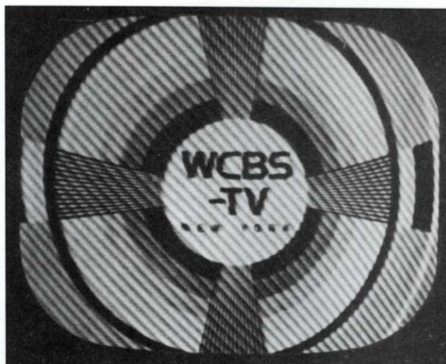
Figure 6.7 — Harmonics radiated from an amateur transmitter may cause "crosshatching."
