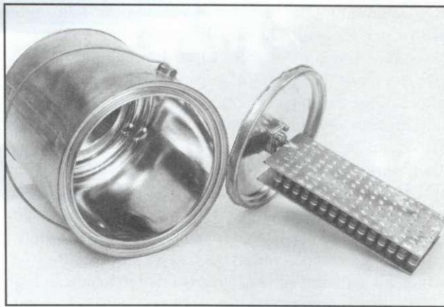
Figure 8.62 —A dummy antenna like this one uses a liquid coolant, often transformer oil, to dissipate heat. Dry dummy antennas dissipate heat into the air.
