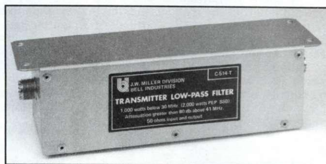
Figure 6.8 — A low-pass filter. When connected in the coaxial cable feed line between an amateur transmitter and the antenna, a low-pass filter can reduce the strength of transmitted harmonics.
