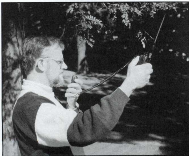
Figure 10.10 — Keep the antenna of a hand-held radio as far from your head (especially your eyes) as possible while transmitting. A remote microphone allows you to hold the radio farther away.
