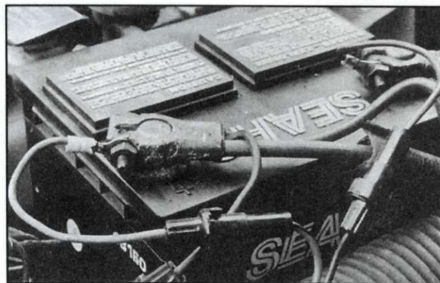
Figure 10.3 — To protect your mobile equipment against being “zapped” install fuses on both the positive and negative leads, close to the battery terminals.
