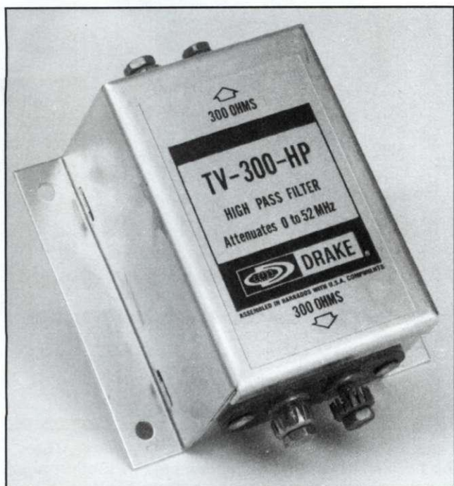
Figure 6.6 — A high-pass filter can prevent fundamental energy from an amateur signal from entering a television set. This type of high-pass filter goes in the 300-ohm feed line that connects the television to the antenna.
