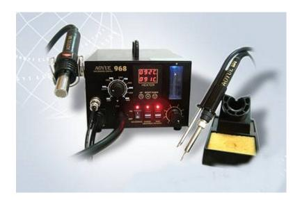
Proffesional rework station AOYUE 968 is an two in one (hotair station with soldering iron with Smoke Absorber buil-in). With this device you can replace any BGA or SMD elements like also normal DIP cover chipsets. This rework station with LCD to precise temperature regulation by microchip (1C skip) and soldering iron from 200C-480C. Beacouse many solder paste generate smoke this station got's build-in smoke absorber to absorb smoke when you are working on PCB board.
