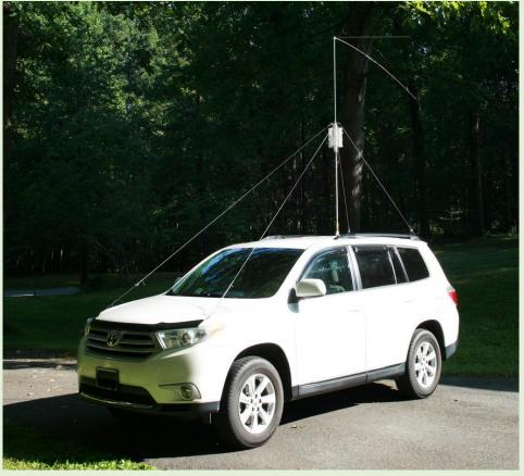
I plan to operate mobile again this year. Bands will be 80 m, 40 m and 20 m; modulation will be SSB. As last year, 80 m will likely be my primary band, even during daylight hours.
