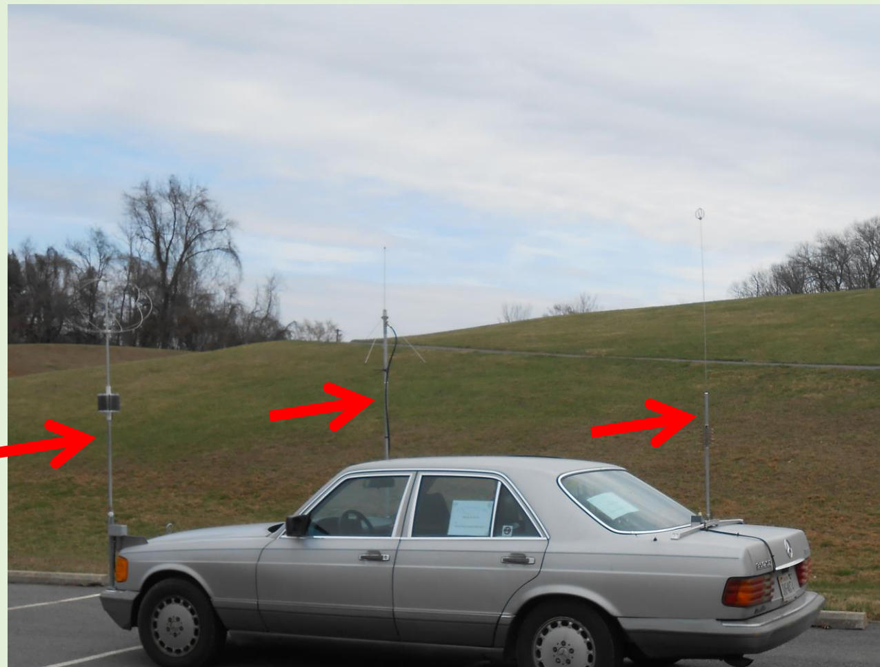
Mobile shown with 2m 10m and 80m home built antennas mounted.
