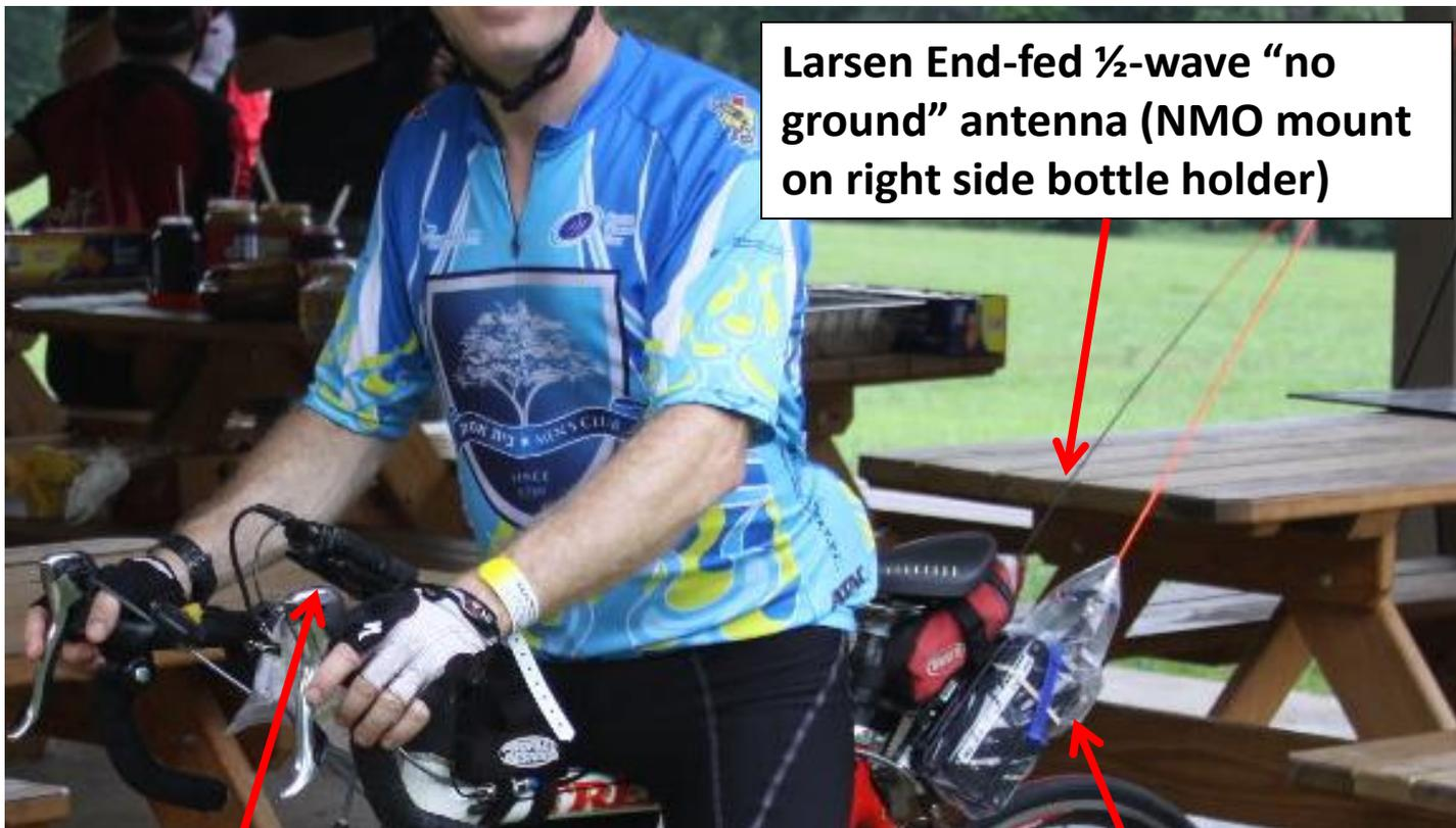
Larsen End-fed ½-wave “no ground” antenna (NMO mount on right side bottle holder)
