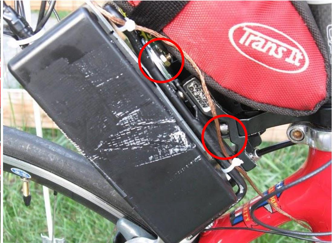
Duct tape field repair after a critical attachment holding the APRS tracker to the bike failed 10 miles earlier when a lock washer didn't (do it's job)!
