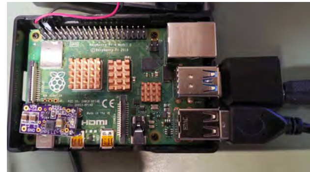
Raspberry Pi 4 with Switching Mode Power Supply for Grape Receiver and GNSS Disciplined Oscillator
