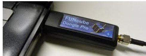
SDR receiver good for satellites, decode weather images
