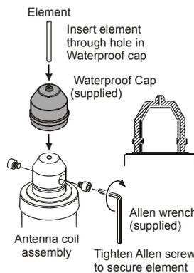
*Note: Installation of the ATAS-120A on a hatchback or trunk lid may not permit a low SWR to be obtained. A solid bond to the car body is important so as to establish a counterpoise for the vertical radiating element.*
