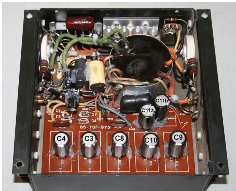
Figure 4 - Chassis Photo (C3/C4/C8/C9/C10/C11a/C11b & D1-D4 replacements annotated)
