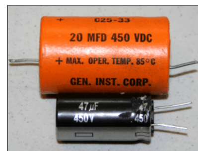
Figure 3 - Electrolytic Capacitors - Then & Now
