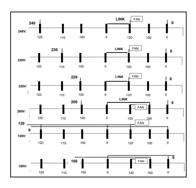
Figure 3: TRANSFORMER AC INPUT CONNECTIONS
