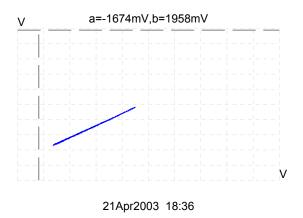
**Fig. 5** Sample of linearity curve obtained on a DX-1d at 750 W PEP output, by using a two-tone generator and a PC oscilloscope in XY mode.
