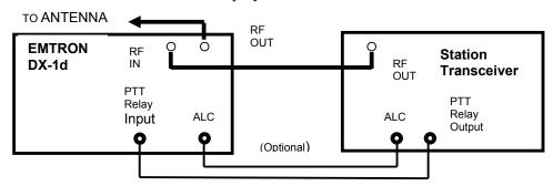
Figure 2. Connections between DX-1d and Station Transceiver
