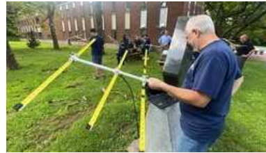
The teachers made tape measure Yagi antennas for the experiment. [Sierra Harrop, W5DX, photo]
