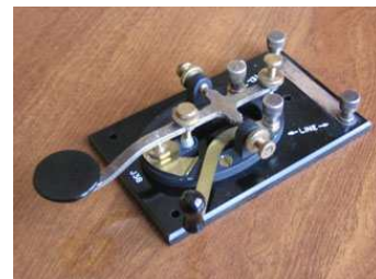
A straight key, like this one from WW2, is still used to day.
