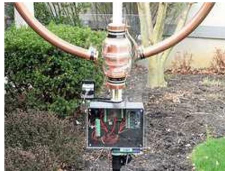
He worked up a reduction drive and remote motorized tuning, and was able to make several FT8 contacts, using his antenna analyzer to tune the loop. “The tuning would shift as I was transmitting,” Robbins recounted. “This is a result of a very high circulating current and heating of
