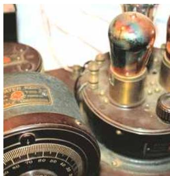
Once a Bakelite product is formed, it will not change shape or melt under heat. In compression molding, the resin is generally combined with fillers such as wood or asbestos before it's pressed into the ultimate product shape. Tube sockets often were constructed using Bakelite. It later found its way into such products as jewelry. In February 1909, Baekeland officially announced his achievement at a meeting of
