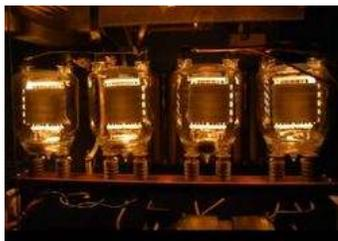
Various stipulations added a level of complexity to the endeavor. First, the transmitter had to be modified as little as possible, retaining original components. The 833 final amplifier tubes (left), better suited for broadcast-band use, would be retained as would the inductance-heavy tuning circuits.
