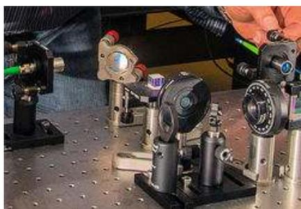
In the NIST tests, the sensor detected digitally modulated magnetic field signals with strengths of 1 picotesla (one millionth of Earth's magnetic field strength) and at frequencies below 1 kHz.
