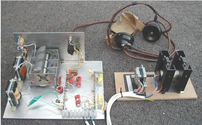
The SAQ broadcasts were received using this RX with my 8 m high, 40 m long inverted L antenna, which produced a comfortably audible signal in the headphones. The limit on sensitivity was the QRN, which was quite strong.
