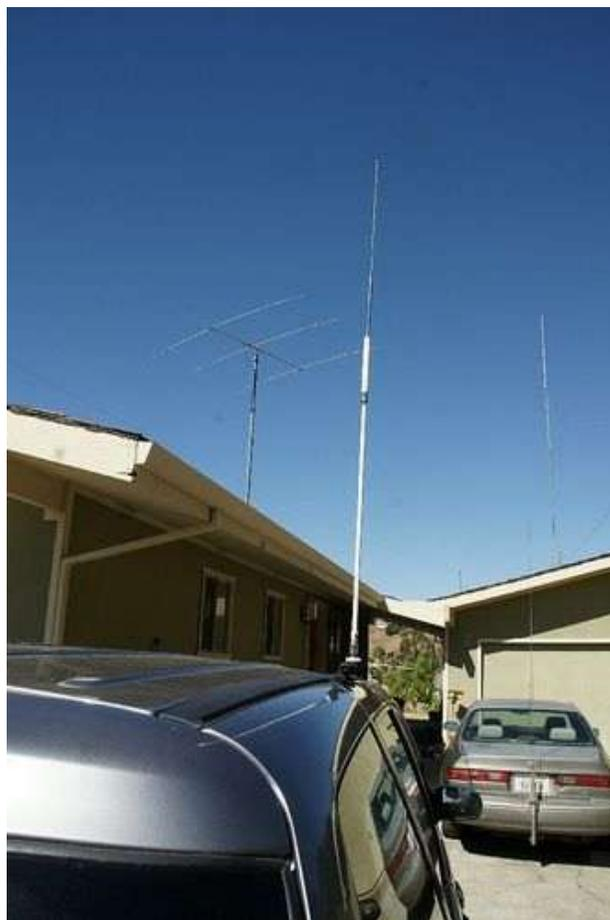
Here you have to attach at the very rear edge, else the sliding closure motion uses the four Allen screws to rip the full length of the door seal. At the back, there is rotation that slams the door closed at right angles to the seal. Once the lip mount was installed I checked with an ohm meter that the Allen screws had penetrated the paint. I touched the outside of the coax and then a bolt head on the door. I also checked the door to the car and somehow this also seemed to be connected.
