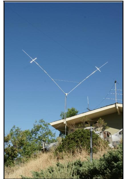
of one in the air and using a slip of paper held against my computer monitor I was able to mark the length of the outboard trap on a piece of paper. Using this as a ruler, I was able to measure the distance to the capacity hats and the length of the adjustable end pieces. The capacity hats were one trap length away and the end pieces were two and a half trap lengths long. Transferring this to the actual antenna was the last step in the assembly.
