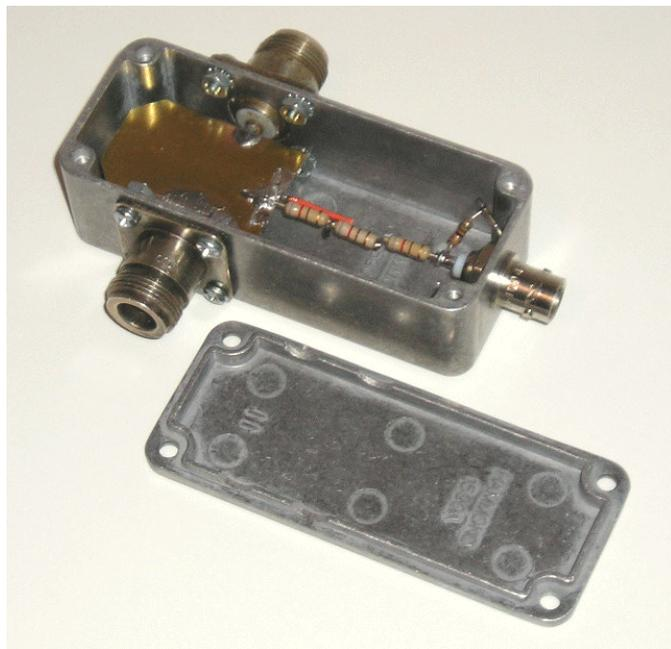
Fig. 2. All of the power tap components are visible in this photo. Note the four notches filed in the cover to clear the N-connector mounting nuts.
