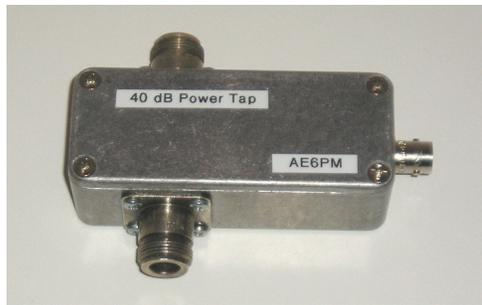
Fig. 1. The completed power tap. The enclosure is 3.64" long x 1.52" wide x 1.06" high.
