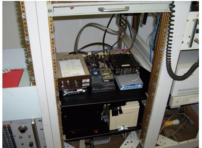
Here's a better look at the middle bay. The rig on the left is for local forwarding on 1.25 M, 10 watts output. The middle rig is the 70 cm 9600 baud user port, 4 watts output. And the one on the right is the 2 M 1200 baud user port, 10 watts output.
