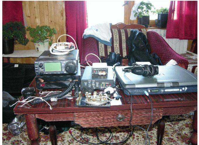
My setup was ICOM 706 MK2G, LDG Z-11 Pro Tuner, Signal link SL-1 sound card interface, random wire antenna, MFJ 33 foot push up mast and HP Omni book laptop. I worked most of Europe, West Asia, Middle East and some DX stations. I worked Siberian and North American East Coast stations. Propagations were pretty good and bands were open almost the whole day and night, but unfortunately not very good for communication with California.
