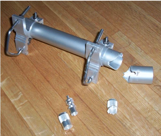
**This is the old antenna base mount. That tubing should be all in one piece! The connector shell on the right should look like the new one on the left, who knows where the rest of it is.**
