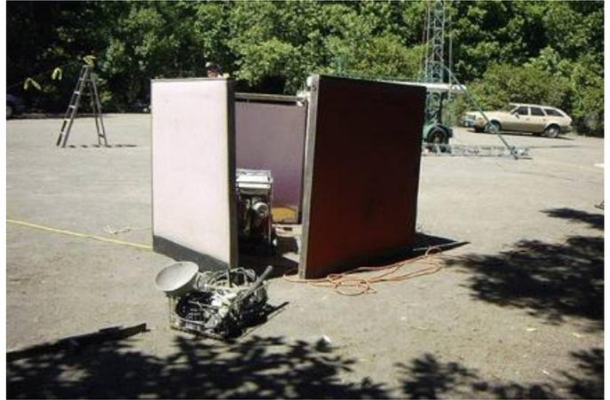
SCCARA's AC generator surrounded by cubicle walls to reduce engine noise. This generator and several DC car batteries supported power needs, SCCARA stations were all based on "emergency power."
