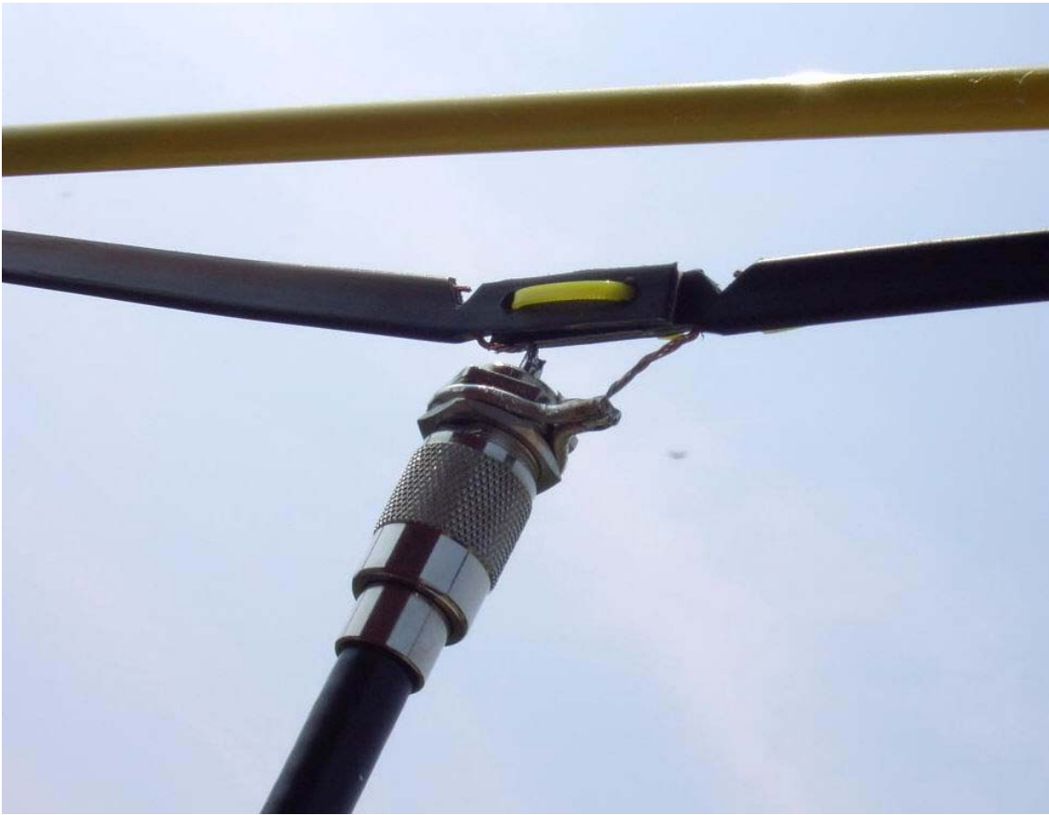
Figure 8c – Connection of 50 \Omega coax to array without a balun.
